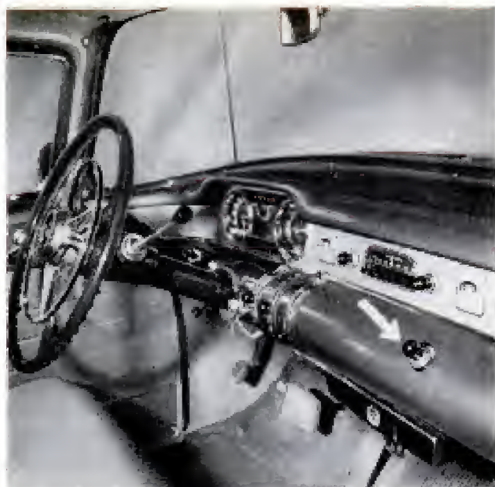
Cigarette lighter protrudes from dash dangerously (arrow). It requires driver to have a long reach
